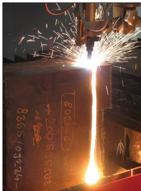
500 mm steel plate cutting
